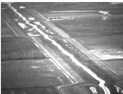
Channelized streams increase gradient and flow speed, eroding streambanks and degrading habitat.
