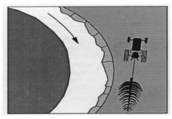
**1.** First tree is moved into place on bank. Arrow shows direction of current.
