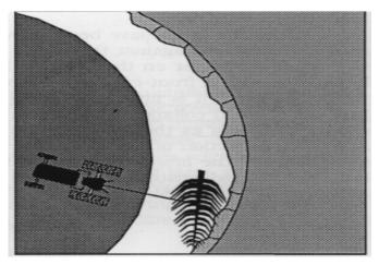
2. Tree is pulled into stream. A tractor with a front-end loader can also be used to drop trees into place.
