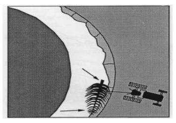
**3.** Tree is pulled tightly against bank and anchored at points shown by arrows.
