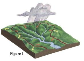
catches snow, rain and other types of precipitation that fall on the land. Then the surface watershed delivers some of the precipitation to the stream. Uplands, floodplains, riparian corridors and stream channels are all part of the surface watershed. Just as important as the surface watershed is the underground area, called the *recharge area* or *groundwater source area*, that delivers groundwater to a stream.
