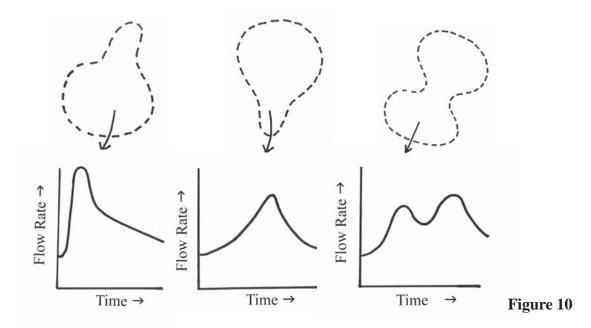
A watershed with a round shape produces fast, high flood peaks because water has a shorter distance to travel from headwaters to mouth. Long, narrow watersheds have longer distances for water to travel and will have more moderate flood peaks (Figure 11).
