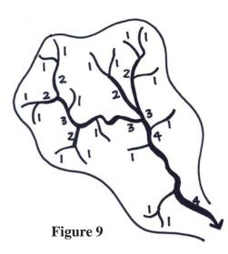
where a first order stream joins a second order stream, the larger stream is still second order stream, not a third order. A third order stream is only created where two second order streams flow together. Two third orders form a fourth order, and so on (Figure 9).
